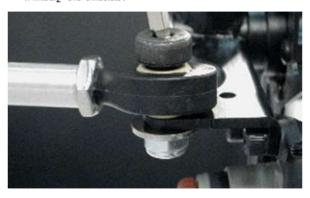
Take the tie rod and turn the jum nuts all the way out towards the rod-end bearings if they aren takeady, then screw the rod-end bearings in as far as they Ilgo. Locate the tie rod bolton each kingpin assembly. Hold the boknutwith an adjustable wrench and remove the bolt, spacer and washer.
