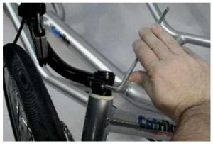
Because we have no control overhow tightly you assemble your Catrike it is extremely important for you to re-check all of the threaded fasteners (pedals, axle bolts, and all other muts and bolts) on the trike after you've ridden it for a couple of hours, just to make sure everything is still tight. Periodic checks during the riding season also are a good idea. Virtually all of the trouble reports we receive are nothing more than fasteners that have worked bose.
