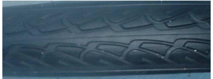
On the tire, the "arrows" point left, giving you direction of rotation.
