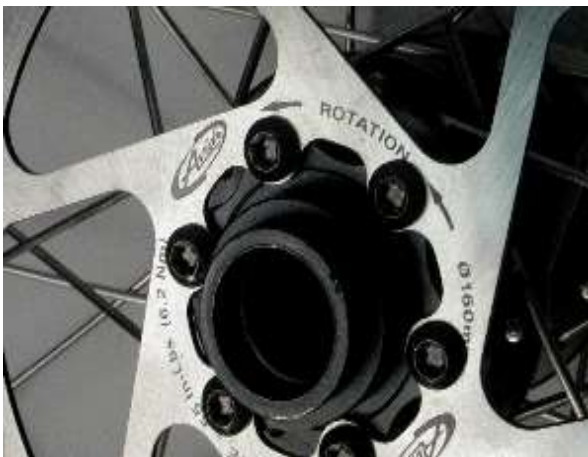
Direction of rotation shown on brake rotors
